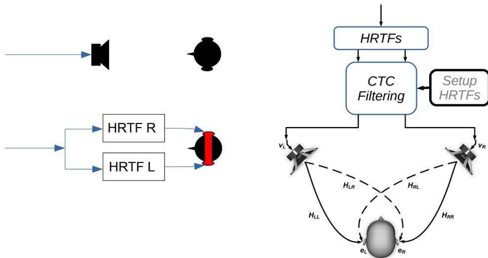
Figure 4: Top left: Free-field sound reproduction via loudspeakers. Bottom left: Binaural synthesis via headphones. Right: Binaural synthesis via loudspeakers.
