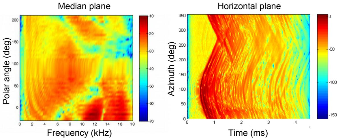
Figure 3: Head-related transfer functions of the left ear of NH5. Left: Amplitude spectra of the directional transfer functions in the median plane. Right: Energy-time curves of the head-related impulse responses in the horizontal plane. The color encodes the amplitude in dB re max.
