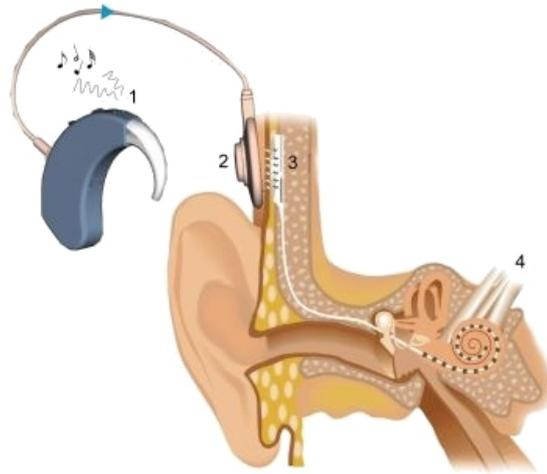
Figure 7: Cochlear implant system. (1) speech processor, (2) transmitter coil, (3) implant, (4) electrode array. From <http://recorlsa.club.fr/implantcochleaire/descripgenerale.html> (29.11.2007).
