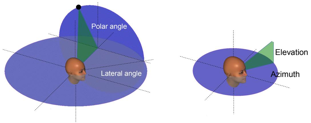
*Figure 2: Left panel: Interaural-polar coordinate system for sound localization in humans. Right panel: geodetic spherical coordinate system usually used in acoustics and mathematics.*
