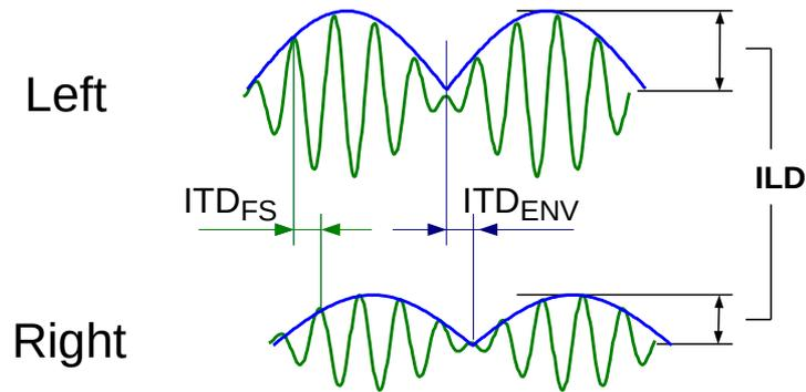
Figure 6: *ILD, fine-structure ITD ( $ITD_{FS}$ ) and envelope ITD ( $ITD_{ENV}$ ) in a modulated stimulus.*
