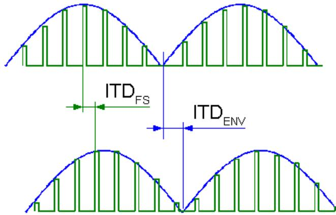
Figure 8: Fine-structure ITD ( $ITD_{FS}$ ) and envelope ITD ( $ITD_{ENV}$ ) in a modulated pulsatile electric stimulus. Only the positive phase of each pulse shown.
